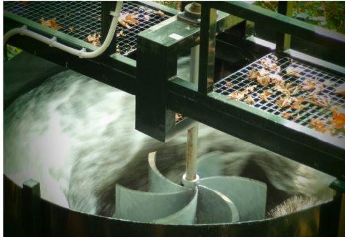
Despite the high output of small-scale hydropower projects (from 500w Pico up to 100kW Micro), they often fail to materialise because of site constraints such as water flow and height differential that render projects unfeasible. Many opportunities have been missed because conventional hydro does not operate efficiently with a fall of less than 3m.
